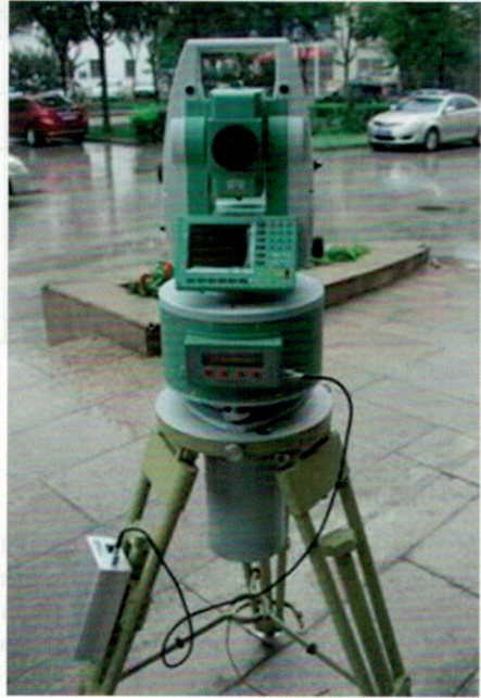
Abb. 22: Automatische Gyro Station BTJ-5vom Beijing Institute of Space Technology, CAS
