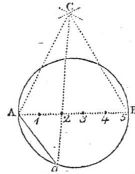
From  $C$ , the apex of the equilateral triangle, draw a line through the *second* division in the diameter, until it touches the circle below, as at  $a$ ; from whence, if a line be drawn to  $A$  (where the numbering began), it will give the length of a side of the required polygon.
