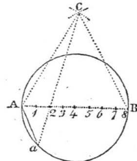
The diameter being divided into 8 parts, draw the line  $C2$ , as before directed, to touch the circumference at  $a$ . Draw  $Aa$ , and it will be the length of a side of the octagon required.
